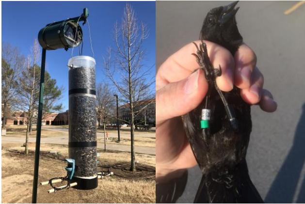
Fig. 1: Bird Feeder with datalogger (A) and a bird banded with a PIT tag (B)
